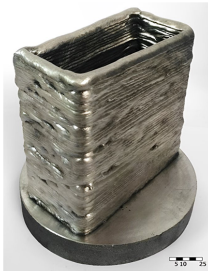
Fig. 12. AZ61 thin-walled object fabricated by WADED.
